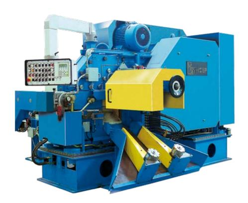
Shears for cutting billets and mechanical bar cutters for cold cutting, hydraulic shears for hot cutting.
