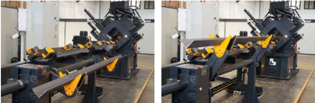
Rotating loading system to transfer the profiles onto the infeed table
