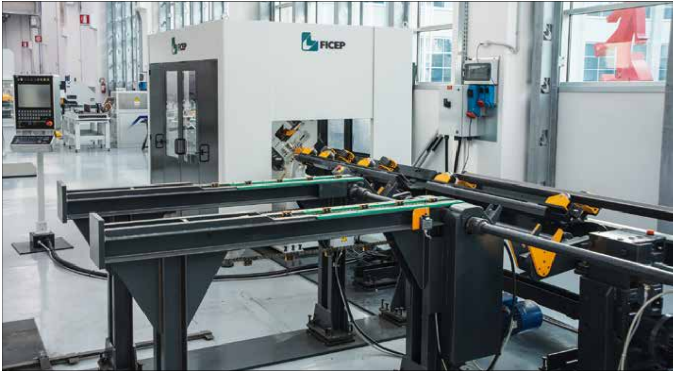
Infeed cross transfer and rotating loading system
