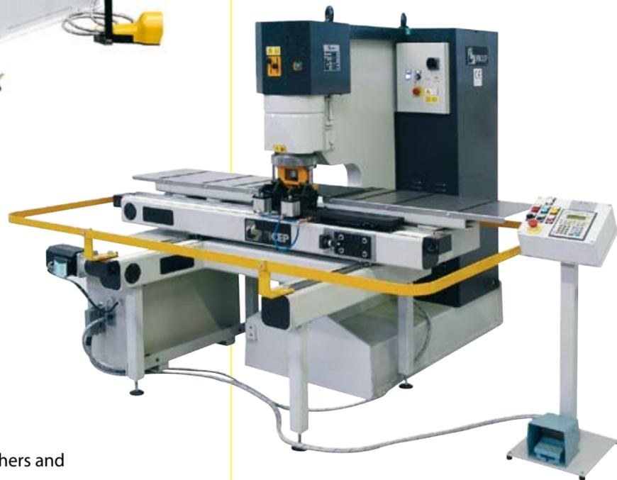
Combined shears and punchers and simple punchers from 400 to 1000 kN.
