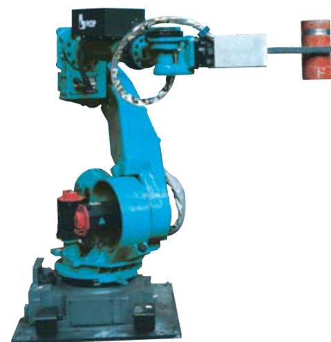
Anthropomorphic robots for automation of steel pressing lines.
