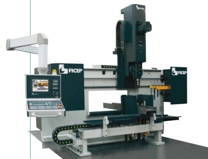
CNC lines for the automatic perforation, marking and cutting of H - I - U sheets, etc.
