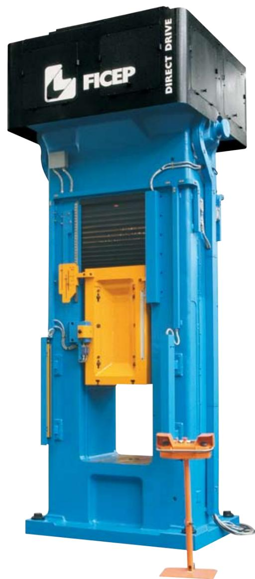
"Direct Drive" screw presses for high-precision hot pressing.
