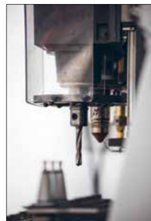
Drilling unit with a 4-position automatic tool changer
