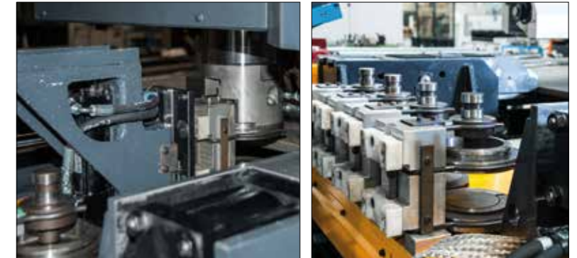
4-position automatic punching tool changer
