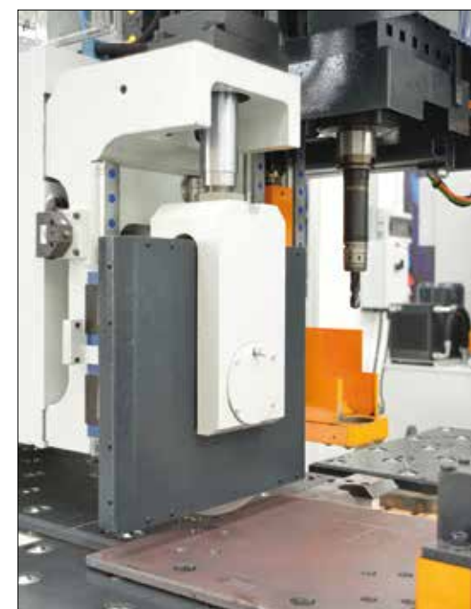
Independent programmable hard stamp marking unit
