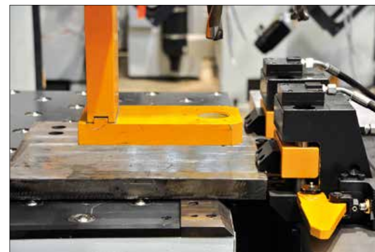
Vertical hold-down and material clamps
