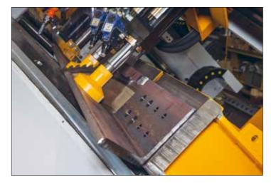
The Tipo D50-F includes with a miter-cutting circular saw with carbide inserts for maximum productivity. The saw can position automatically for miter cuts of up to 60° in either direction.
