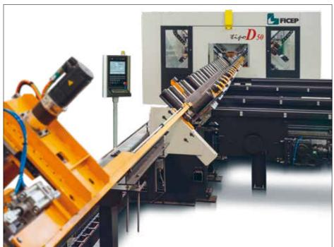
Stock material positioning and measuring into the Tipo D50-F is accomplished with a positive rack and pinion system. Once the clamping of the material is confirmed, the stock length is automatically measured prior to the start of the fabrication process.
