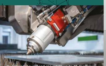
Its optional bevel head can rotate up to 45 degrees in both cutting directions, and also offers an automatic nozzle changer.
