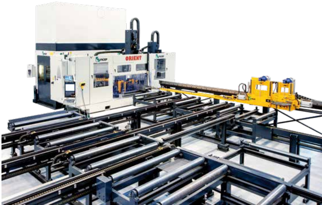
Orient drilling line combined with oxy-fuel/plasma cutting capability
