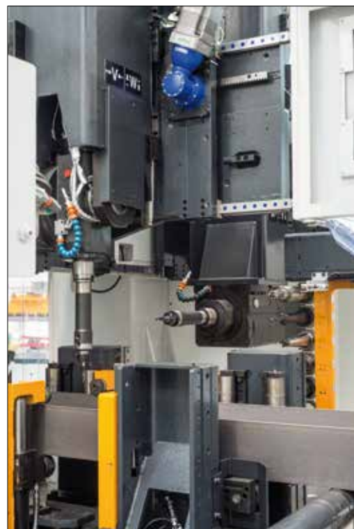
Optional second drill head with automatic tool changer
