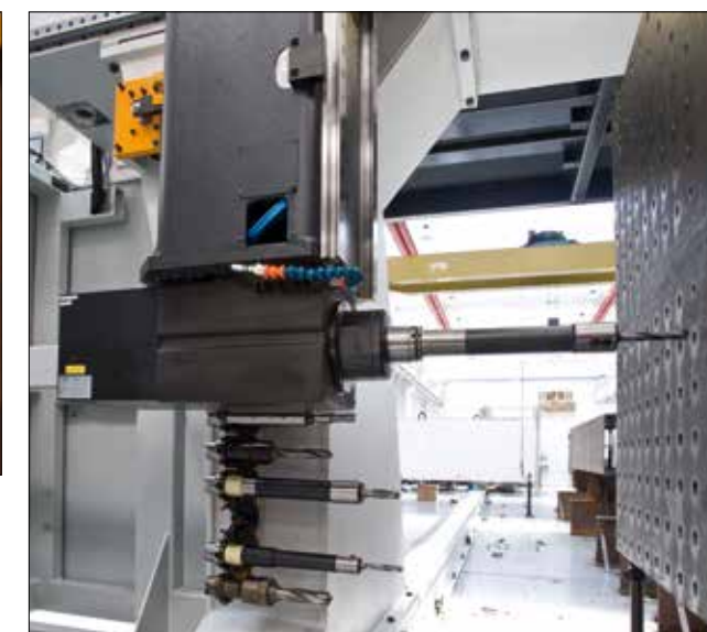
Horizontal spindle with automatic tool changer
