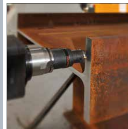
Rotating drilling head for end milling
